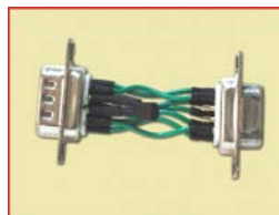
Fig. 4 Illustration of a straight through in-line cable adaptor with DS2401 Electronic tag chip.
